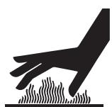
**DO NOT** open the strainer pot if pump fails to prime or if pump has been operating without water in the strainer pot. Pumps operated in these circumstances may experience a build up of vapor pressure and may contain scalding hot water. Opening the pump may cause serious personal injury. In order to avoid the possibility of personal injury, make sure the suction and discharge valves are open and strainer pot temperature is cool to touch, then open with extreme caution.
